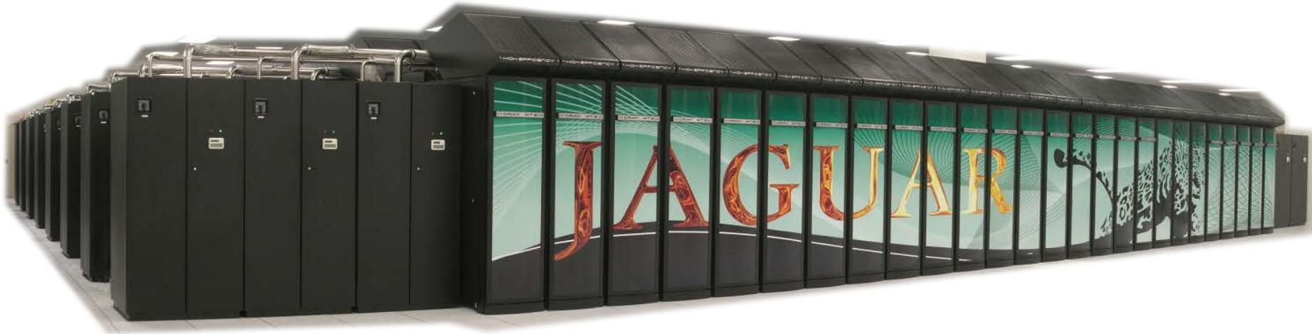
37,360 AMD Operton CPUs, 6 cores/CPU → 224K cores
